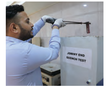
Jominy End Quench Test
